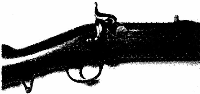
Plate 24. The breech area and backsight of the Heavy Navy Rifle of 1840. Beautifully made throughout, the browned twist barrel is 32 5/8-inches long, and .796" calibre, with the Brunswick two-groove rifling making 1 turn in the length of the barrel. Note that the trigger guard bow is not pierced for a sling swivel screw. Courtesy W. S. Curtis.
